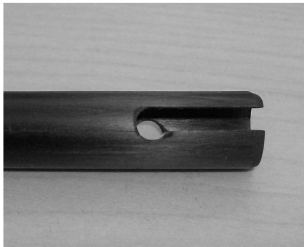
Figure 28. Carbon Fiber Tube Failure
